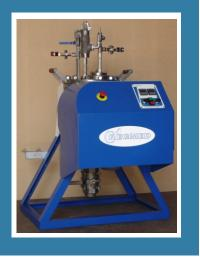
The laboratory reactor model HB-21 has been designed for pilot chemical, semi-chemical and thermal pre-treatments of several types of biomass .
