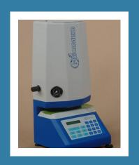
The air permeance of papers has a major importance in the specification of materials for the packaging and printing industries. The air permeance is the flow of air through unit area under unit pressure difference in unit time, under specified test conditions and is expressed in  $\mu m/(Pa.s)$ .
